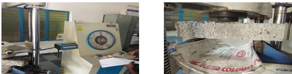
Fig 1.3 Flexural Strength of Concrete
