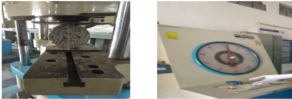
Fig 1.2 Split Tensile Strength of Concrete
