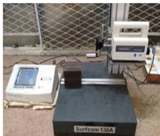
Fig 2.4: Surface roughness measuring instrument (Surfcom 130A)
