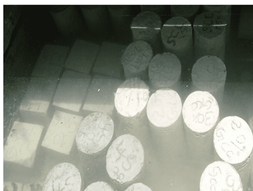
Fig 12 Curing of Specimen
