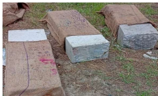
Fig 15 Curing of Beam
