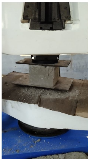
Fig.11 Cube Under Compressive Load
