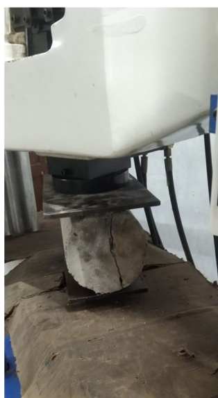
Fig. 12 Cylinder Under Tensile Load
