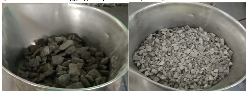
Fig.3 Coarse aggregates of 20mm and 12.5mm
