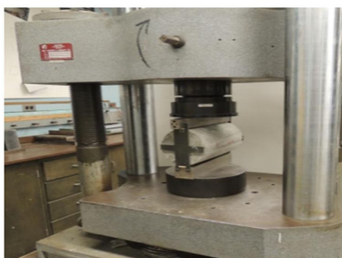
Split tensile strength setup
