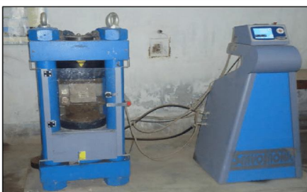
Automatic Compression Testing Machine (MATEST s.r.l.)
