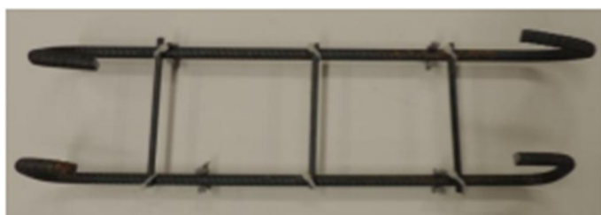
Reinforcement and Framework for RFC Beam
