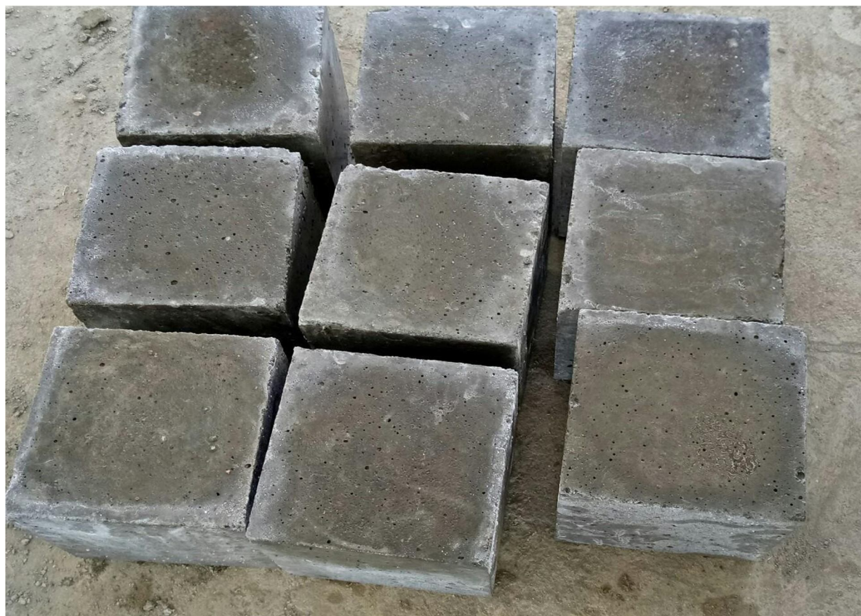
Fig.3 - Cubes for testing
