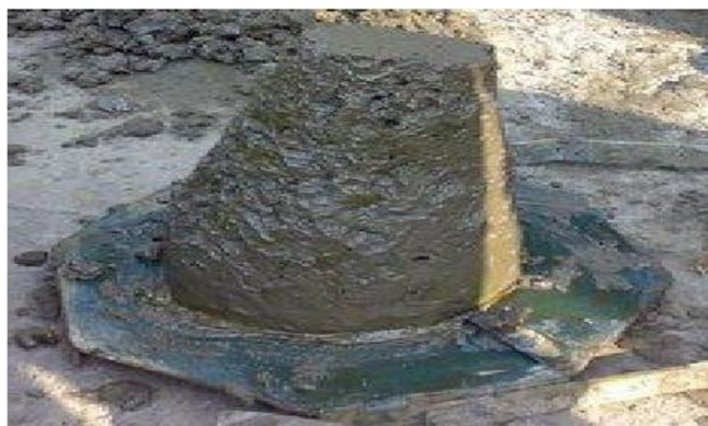
Fig. 6 - Slump cone test in progress
