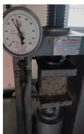
Figure 6- Compressive Strength Test of Concrete Cube
