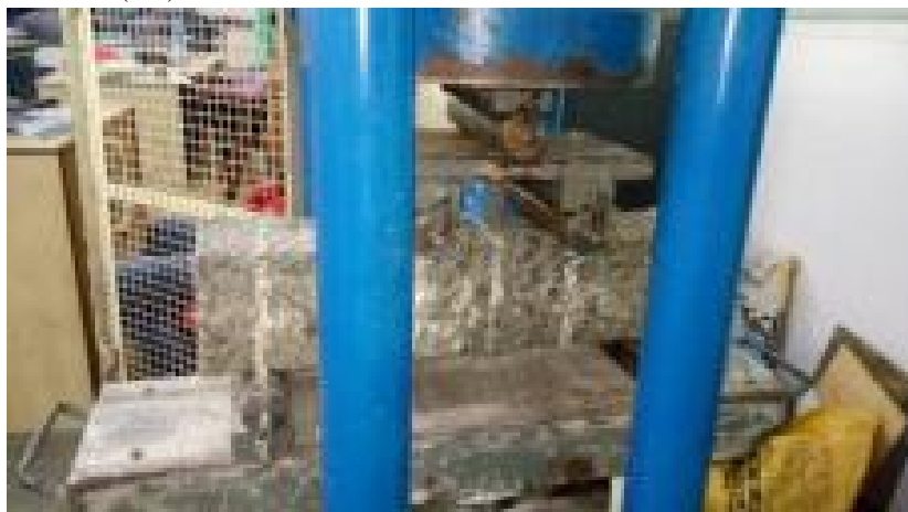
Figure 3: Flexural strength test without fiber
