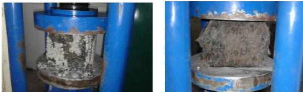
Figure 2: Cubes with fiber and without fiber
