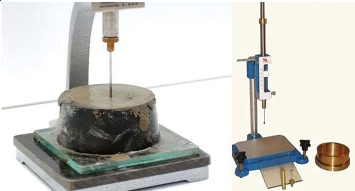
Fig. 5 Initial and Final Setting Time of Cement
