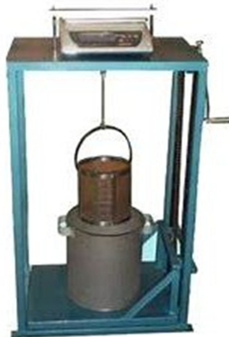
Fig.8. Water Absorption test apparatus
