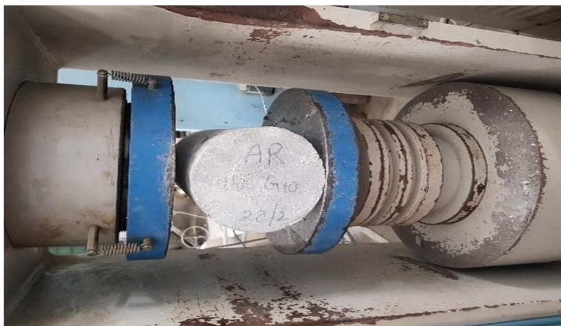
Fig.28. Testing of cylinder in Compressive strength testing machine
