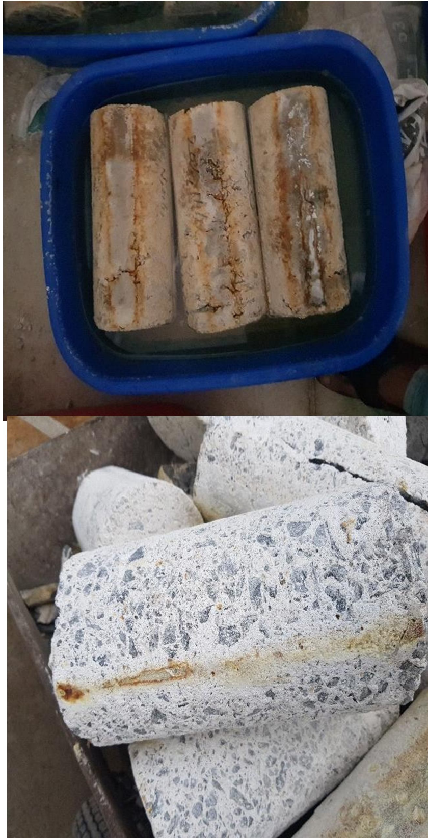
Fig: Effect of 1% of Sulphuric acid on M30 grade concrete cylinders
