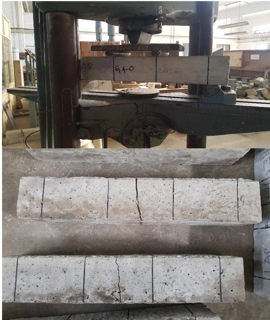
Fig.29. Testing of prism for flexural strength
