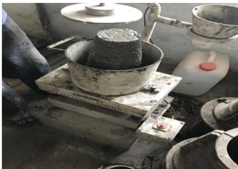
Fig: Vee-Bee Consistometer Test Procedure for Vee-Bee Consistometer Test
