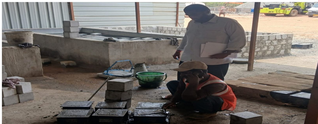
Fig.17. Casting of Cubes
