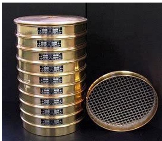
Fig.15. Set of Sieves for fine aggregate
