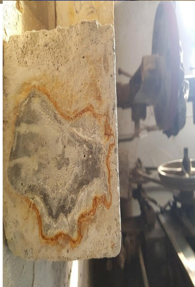
Fig: Effect of 1% of Sulphuric acid on M30 grade concrete cubes
