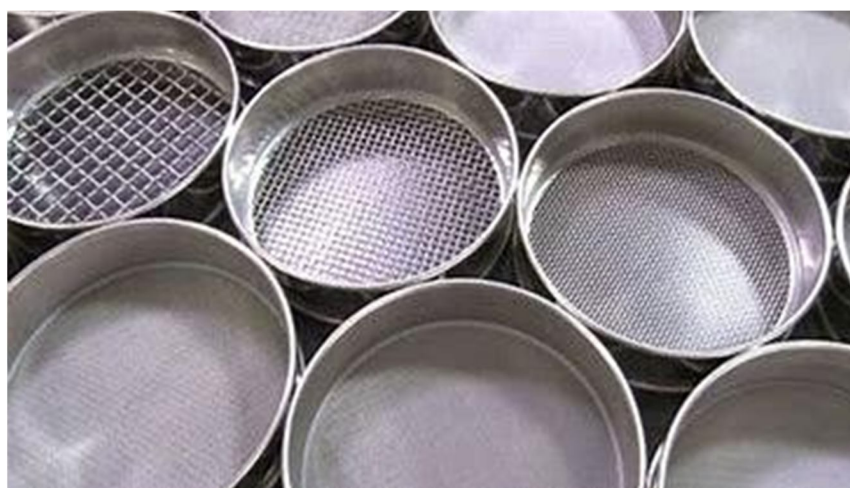
Fig.16. Set of Sieves for coarse aggregate
