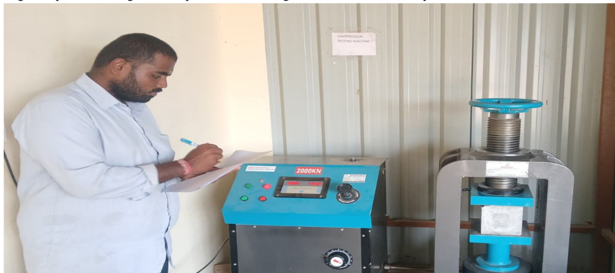
Fig.27. Testing of cube in compressive strength testing machine
