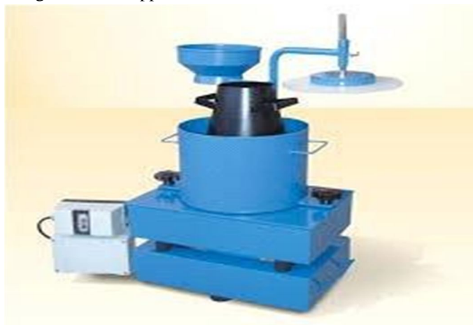
Fig.24. Vee-Bee Consistometer apparatus
