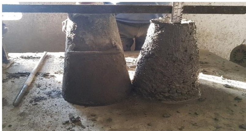
Fig.22. Slump Cone Test
