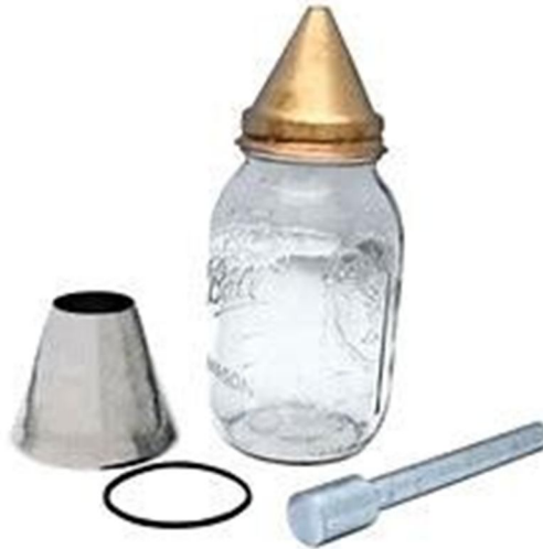
Fig.16. Specific Gravity apparatus
