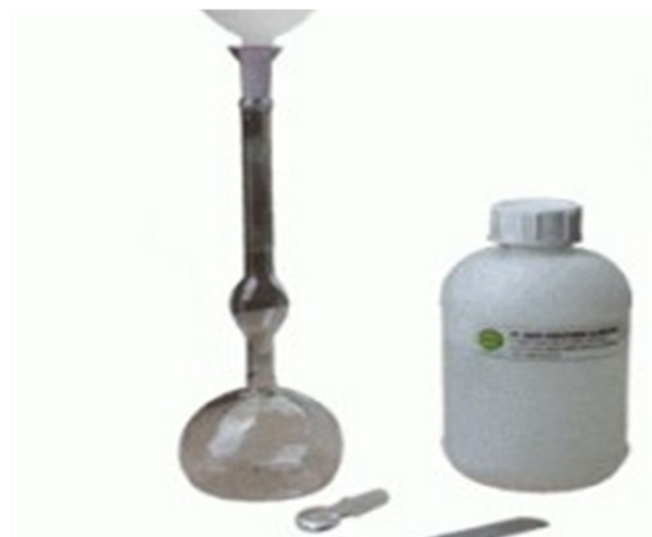
Fig.2. Specific Gravity Apparatus
