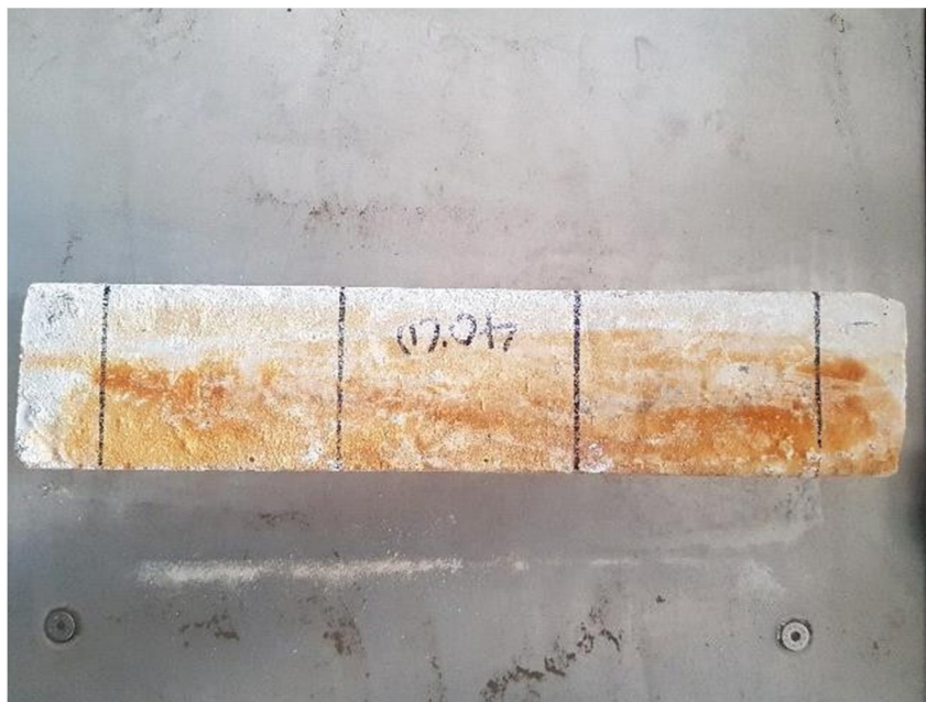
Fig: Effect of 1% of Sulphuric acid on M30 grade concrete prisms
