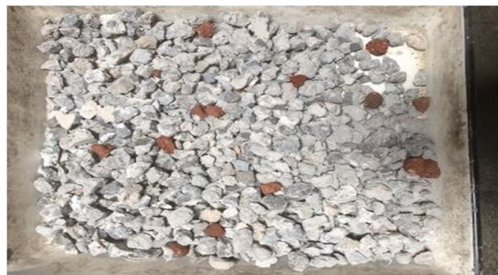
Fig. No. 3.4: Recycled coarse aggregate
