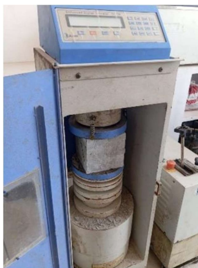
Fig 2: Cube under Compression Test
