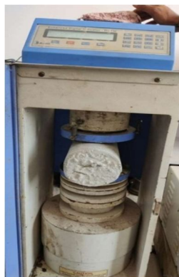
Fig 3: Cylinder under split tensile test
