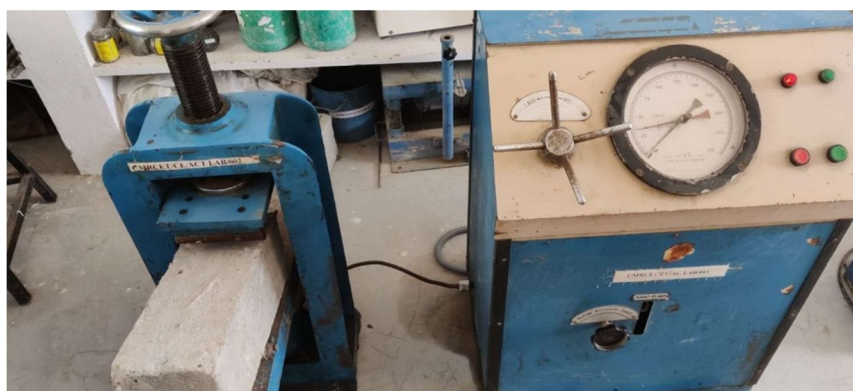
Fig 4: Beam under flexural strength testing machine
