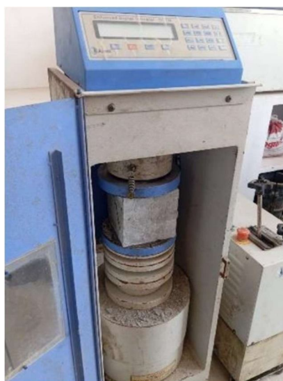
Fig 2: Cube under Compression Test
