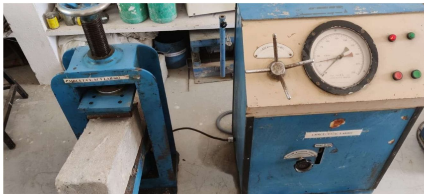
Fig 4: Beam under flexural strength testing machine
