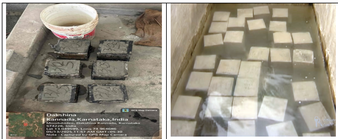
Fig. 4 Casting of concrete in Moulds and Curing of concrete cubes
