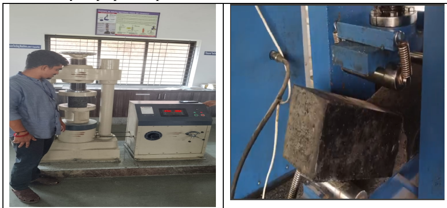
Fig. 2 Compressive and Flexural Strength Test Setup for Concrete Specimens
