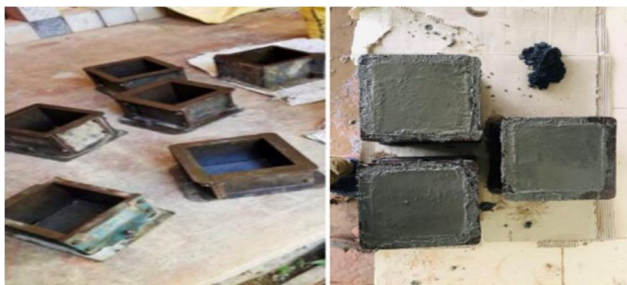
Fig. 2 Casting Mould and Casted Cube
