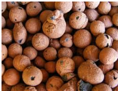
Fig 1: Light weight expanded clay aggregate
