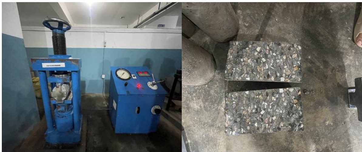
Fig 7: Split Tensile Strength Test
