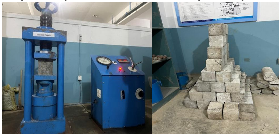
Fig 6: Compressive Strength Test
