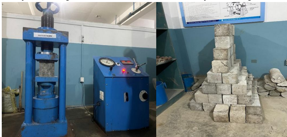
Fig 6: Compressive Strength Test
