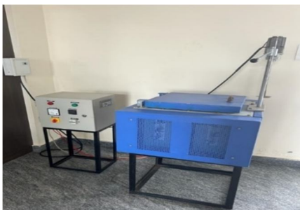
Figure 3.1: Stir casting setup
