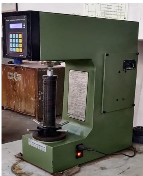
Figure 4.4: Rockwell hardness testing machine
