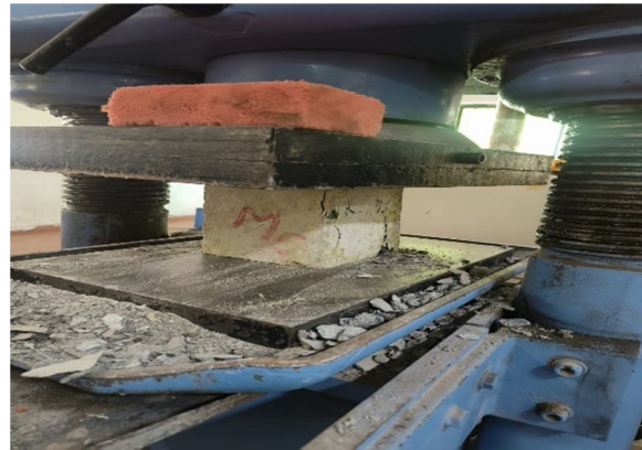
Fig. 2 Compressive Strength Test
