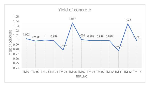
The below graph shown in Fig.No3 illustrates yield of fresh concrete of each trial mix. It has observed that yield of concrete is varies in between 0.977 to 1.037. It shows that in spite of replacing cementitious in various percentage in concrete it is not making drastic change in yield of concrete.
