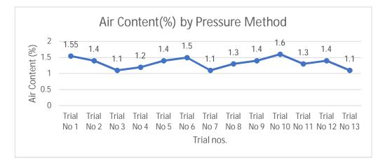
Referring to the above test results it has been found that in GGBFS mix air content vary from 1.2% to 1.6% and maximum air content found is 1.6%. In Flyash concrete the air content varies from 1.1% to 1.4%. It shows that maximum air content found is 1.4%. Air content present in fresh concrete with respect to trial numbers. It has observed from above graph air content is lies between 1.1% to 1.6%.
