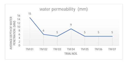
Water permeability test result found more in control mix that is Average Depth of water penetration is 15mm.altough as per DIN 1048 it is less than maximum allowable limit that is 20mm, but it is highest amongst all mixes. Considering other mixes TM03,TM05,TM06 and TM07 Average Depth of water penetration found 5 mm. that is less compare to all other mixes. OPC replacement with GGBS and Flyash both shown exceptionally good resistance to Water permeability.
