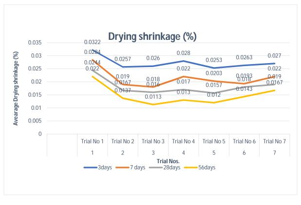
Shrinkage is the inherent properties of cement and concrete. As heat of hydration process takes place and same time concrete start to set. As initial setting time starts the shrinkage activity also starts to stop shrinkage need to retain moisture on concrete surface. The below graph Fig.No. 20illustrate average Drying shrinkage test result at 3,7,28& 56<sup>th</sup> day. More shrinkage observed 0.0322% in TM no 01 at 3rd day. And less shrinkage observed 0.0113% in TM no 3at 56<sup>th</sup> day.
