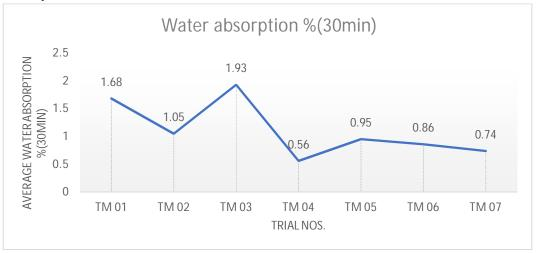
The above graph shown average of water absorption test result at 56th day. The maximum water absorption is observed in TM no 03 that is 1.93% and minimum water absorption observed in TM no 04.that is 0.56%. It shows that Tm no 03 has more water absorption and TM no 04 has less water absorption.
