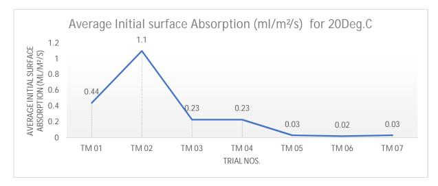
The above graph represents average value of Initial surface absorption at 56th day Highest ISAT observed in TM02 that is 1.1ml/m2/sec. and lowest ISAT observed in TM 06 that is 0.02ml/m2/sec. That mean trial no 06 has less absorption compare to all other result. ISAT value may increases due to porous concrete surface or high water absorption of raw material used in concrete mixes.
