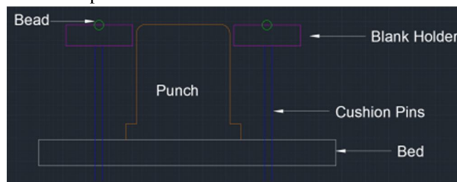
Fig. 5. Conceptual drawing of draw bead
