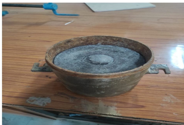
Figure 1(c): CBR Test Result
