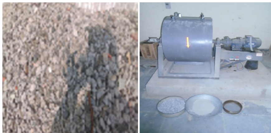
Figure 1 Mechanical Treatment on recycled coarse aggregate
