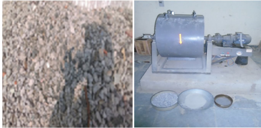
Figure 1 Mechanical Treatment on recycled coarse aggregate
