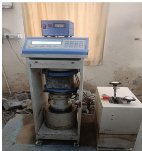
Fig 2 - Testing of compression strength cube.
