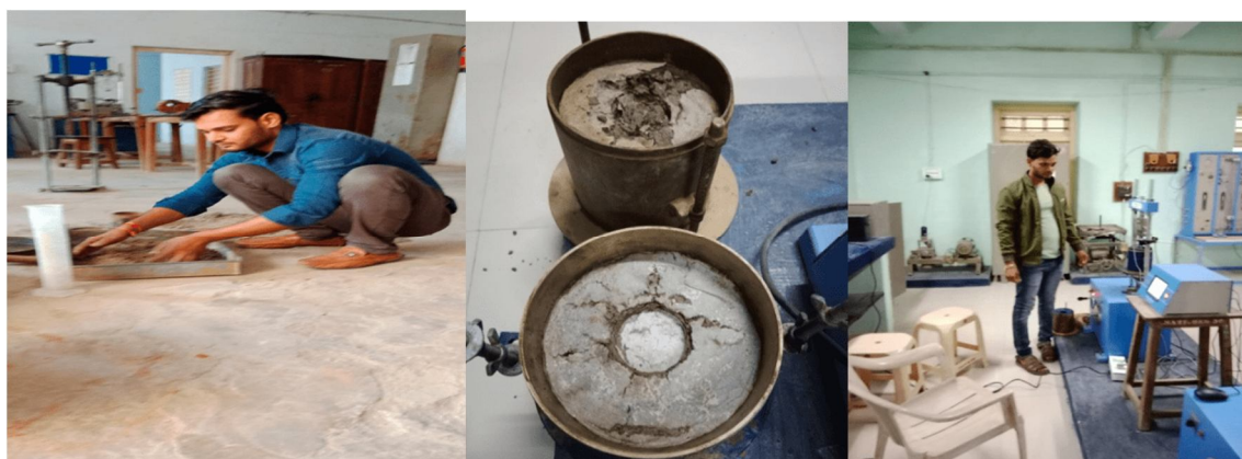
Figure 3.CBR Test in Laboratory
