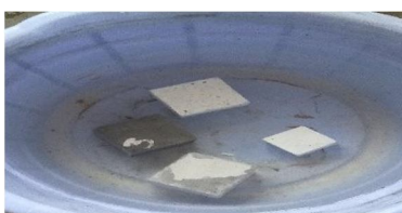
Figure 7: Chloride Attack of Bricks
