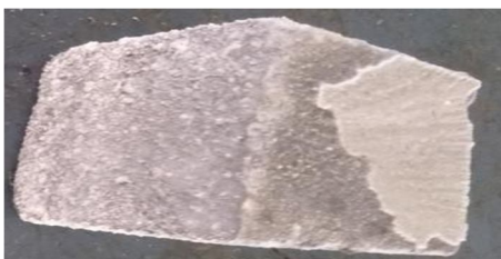
Figure 6: Sulphate Attack of Brick
