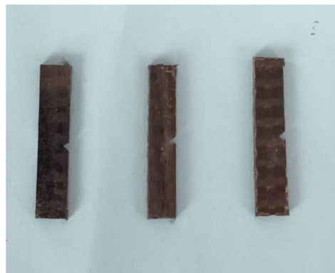
Fig. 7 Specimen section according to ASTM D256
