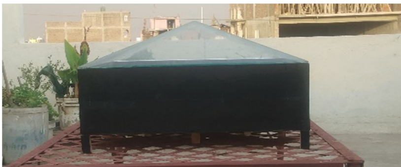
Fig. 1 Pyramid type solar still for experiment.
