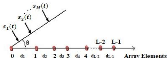
Fig. 1 Array signal model
