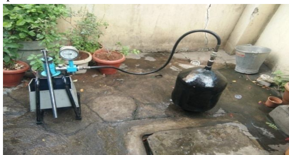
Fig-10: Hydrostatic testing of pressure vessel
