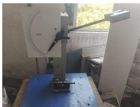
Fig 14: Impact testing on IZOD impact equipment
