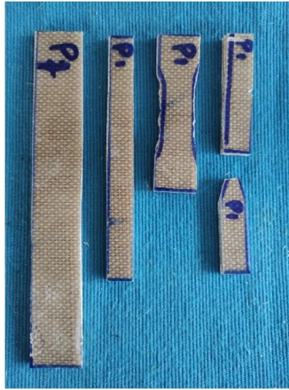
Figure 10: Final composite (Cut into test specimen)
