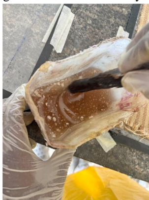
Figure 8: Mix PLA in Resin
