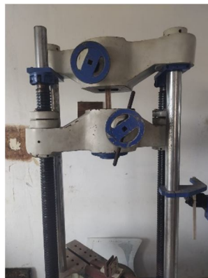
Fig 12: Compression test on UTM
