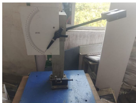
Fig 14: Impact testing on IZOD impact equipment
