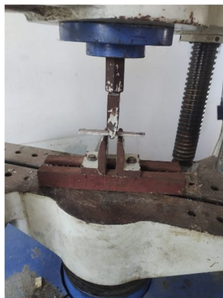
Fig 13: Flexural test at UTM
