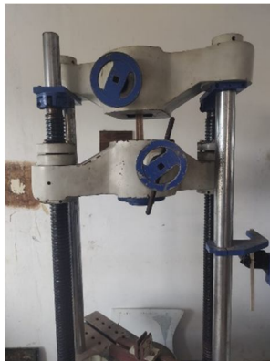
Fig 12: Compression test on UTM
