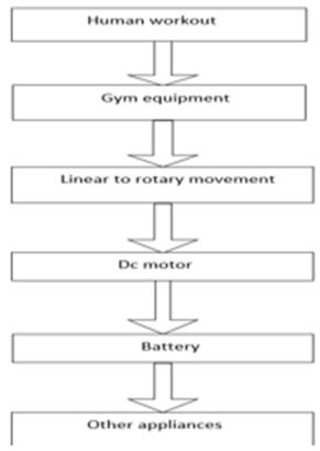
The system provides resistance to the reciprocating movement with the help of springs while generating power. Due to this resistive motion, the system has a greater tendency to restore back to its original position with minimum loss in energy.
