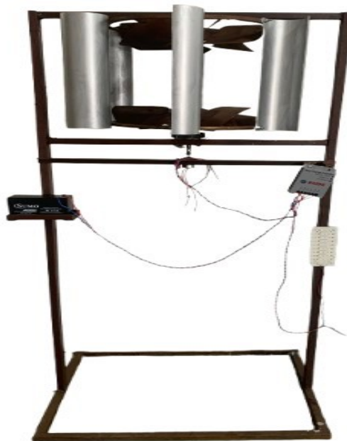
Figure 1- Actual Image of fabrication of levitating frictionless vertical windmill'
