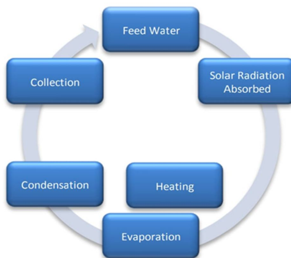
Fig1: Flow chart on process of Distillation
