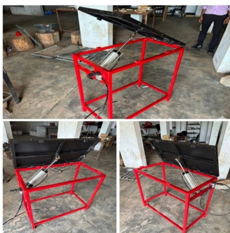
Figure 15: Trailer Tilting Towards Rear, Left and Rear Side
