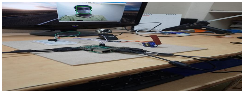
Fig5: Mask is detected door is Open using servo and the LED is on and after 10 sec the door automatically closes and goes off
