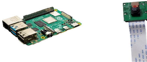
Fig -1: Raspberry Pi 4 and Pi-Cam
