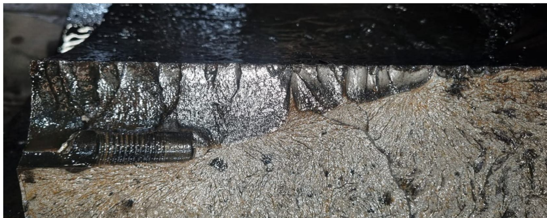
Fig.4 Fatigue crack initiation nearby wear pad of sleeve
