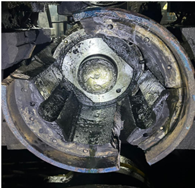
Fig.2 Sleeve found cracked at 3 nos of location
