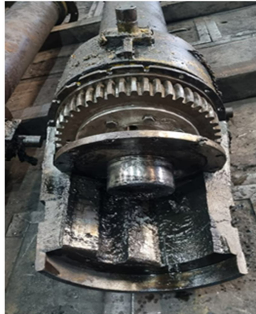
Fig.3 Cracks found nearby wear pad zone
