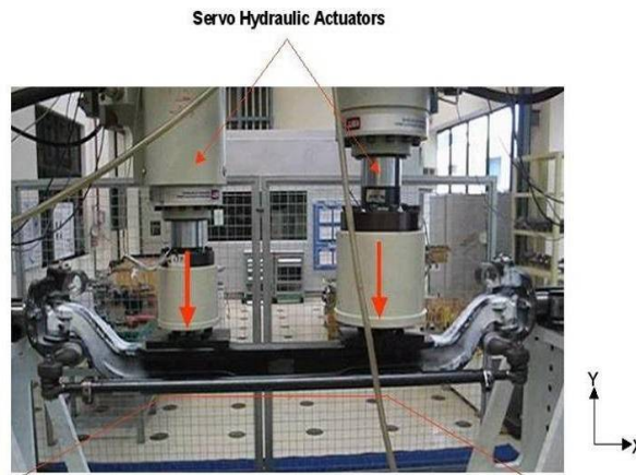
Fig:-Fatigue Loading Testing Setup
