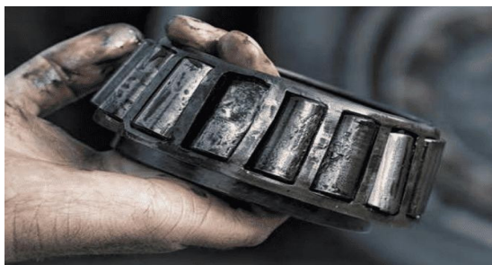
Fig Improper Lubrication and Fretting
