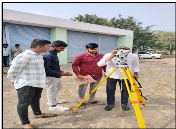
Fig.no.1. Calculation of head with the help of the total station.
