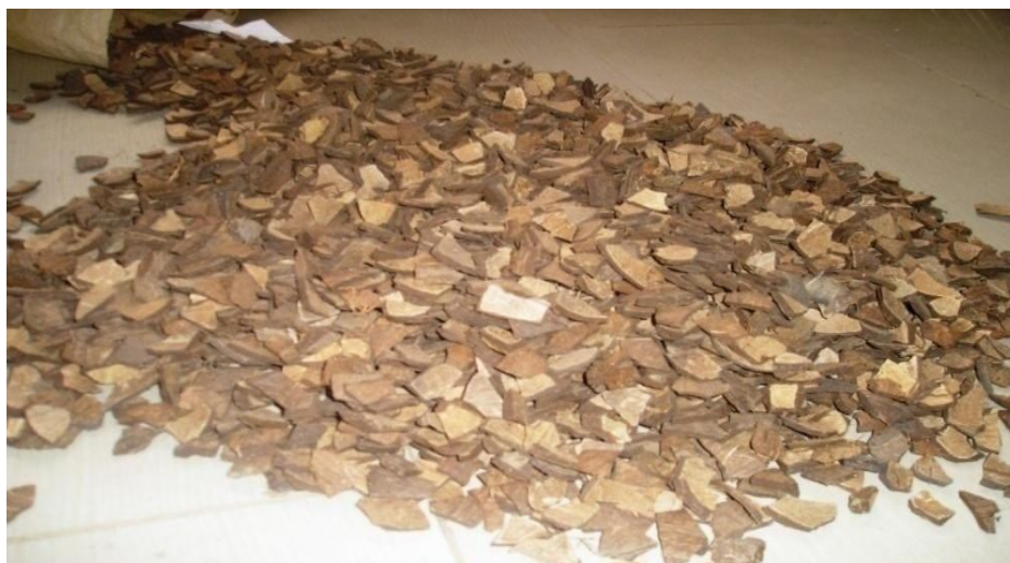
Fig 6. Machine crushed Coconut shell aggregate.
