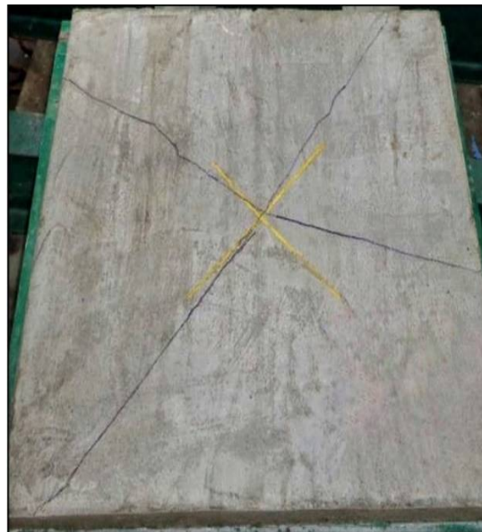
Fig. 4: Crack Pattern in slab
