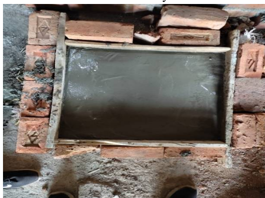
Fig. 2: Slab cube casted
