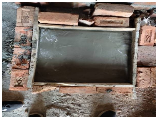
Fig. 2: Slab cube casted
