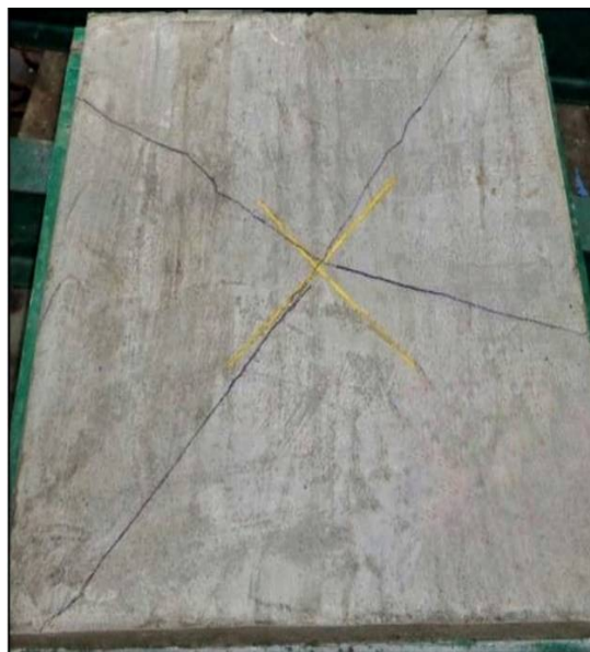
Fig. 4: Crack Pattern in slab
