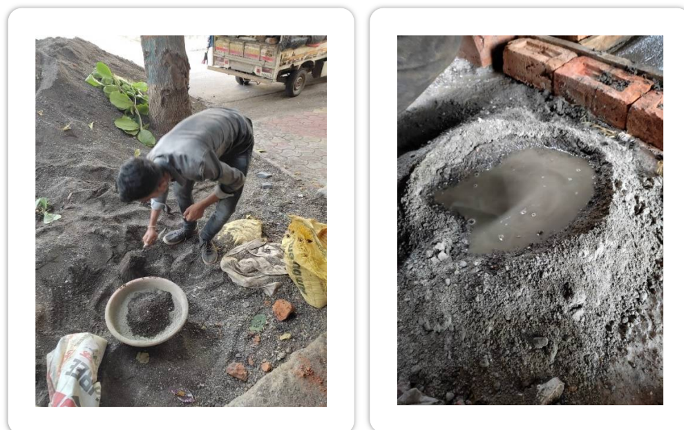
Fig. 1: Process of casting slab cube
