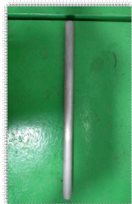
Fig. 1 Mg AZ31B alloy workpiece
