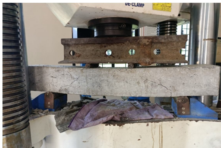
Figure 2 – Test Setup for Flexural test
