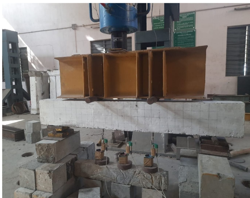
Fig. 2 Experimental Setup for Beam Specimen
