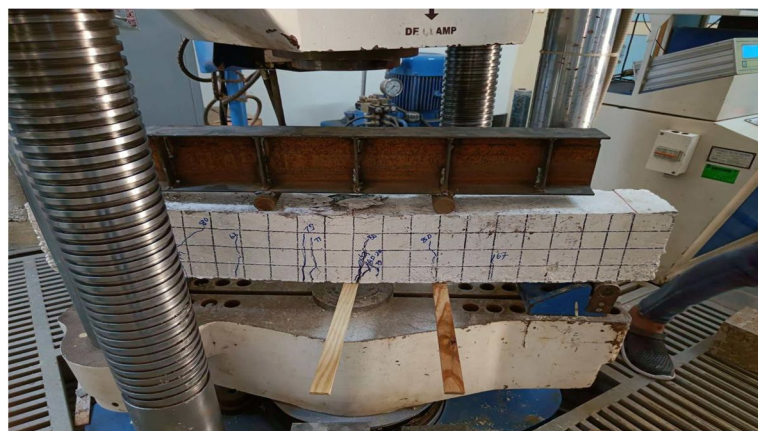
Figure 18 Flexural Test of 10% Replacement Beam
