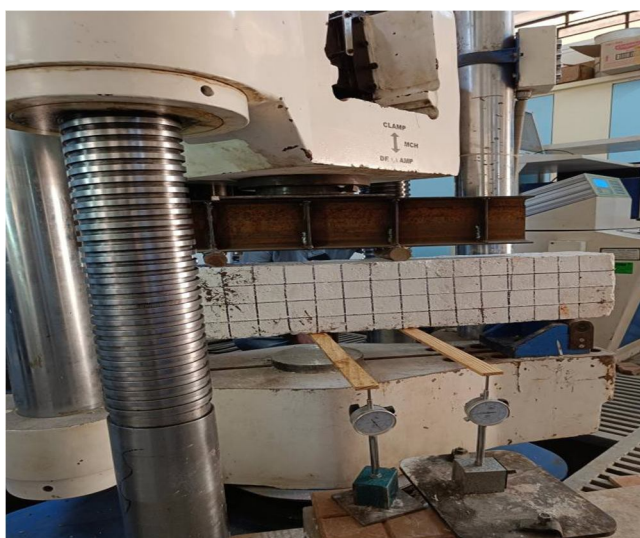
Figure 20 Flexural Test of 15% Replacement Beam
