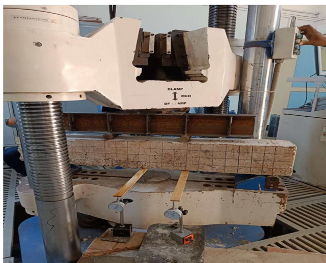
Figure 15 Flexural Test for 5% Replacement Beam
