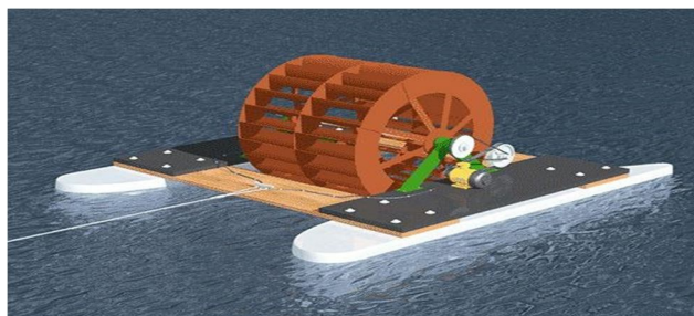
Figure 3. Shows the concept of floating waterwheel power generators
