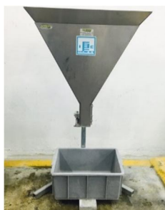
Fig. 3: V-Funnel test apparatus
