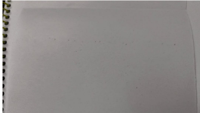
Figure 5.1: Visible Ink Transfer Showing on the A4 paper by Gel pen
