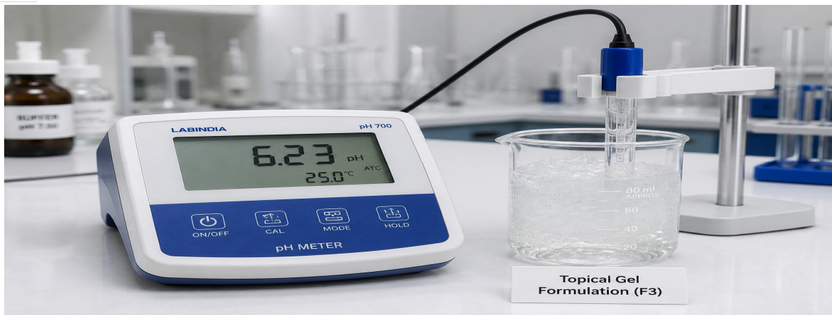
Figure 5 Measurement of pH of optimized topical gel formulation using digital pH meter
