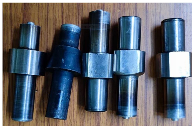
Figure. 4 Friction stir weld tool with various shoulder images
